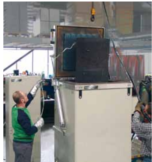
SU 380/06/VA · Furnace for annealing springs in baskets
