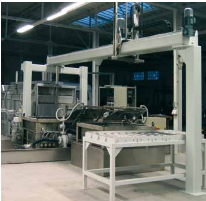
Fully-automatic system Based on a 4-chamber continuous furnace with integrated quenching and washing facility, fully-automatic batch feeding and batch transport, professional process control with extensive documentation options.
