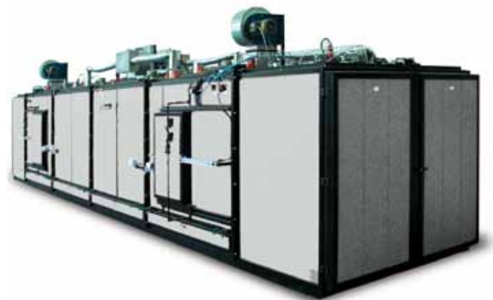
Monorail conveyor furnace DT 34000/02/AS Useable dimensions (mm): 2250 wide x 10000 deep x 1500 high Monorail length 18 m For hardening composite materials With extraction fans for removing vapours
