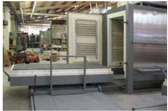
WM 4500/12/S Bogie-hearth furnace with parallel bogie loading system
