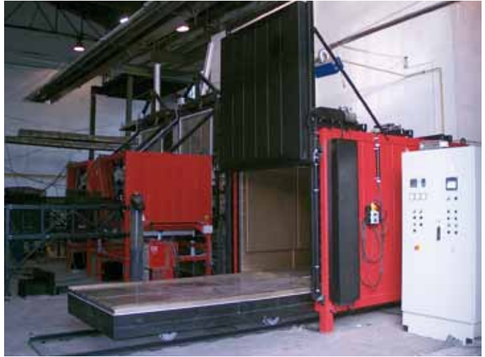
WM 7200/06/A · Bogie-hearth furnace with hydraulic lifting door
