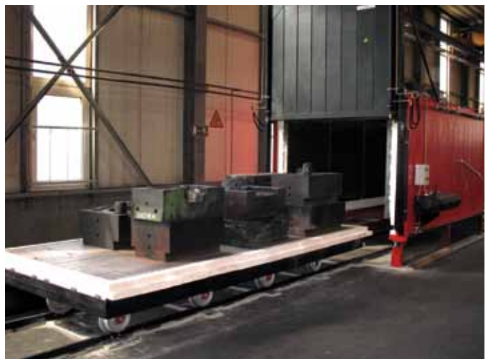
WM 10000/06/AS · Bogie-hearth furnace for 20-tonne charging weight
