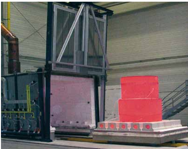
WM 8000/11 GAS Bogie-hearth furnace for annealing steel rings, fitted with reduction system
