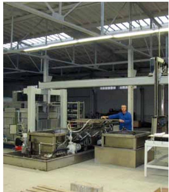
Integrated quenching and washing baths Double quenching bath with circulation pump for different quenching liquids, with automatic drive, baths and collecting tank made of stainless steel, with washing facility and transfer station
