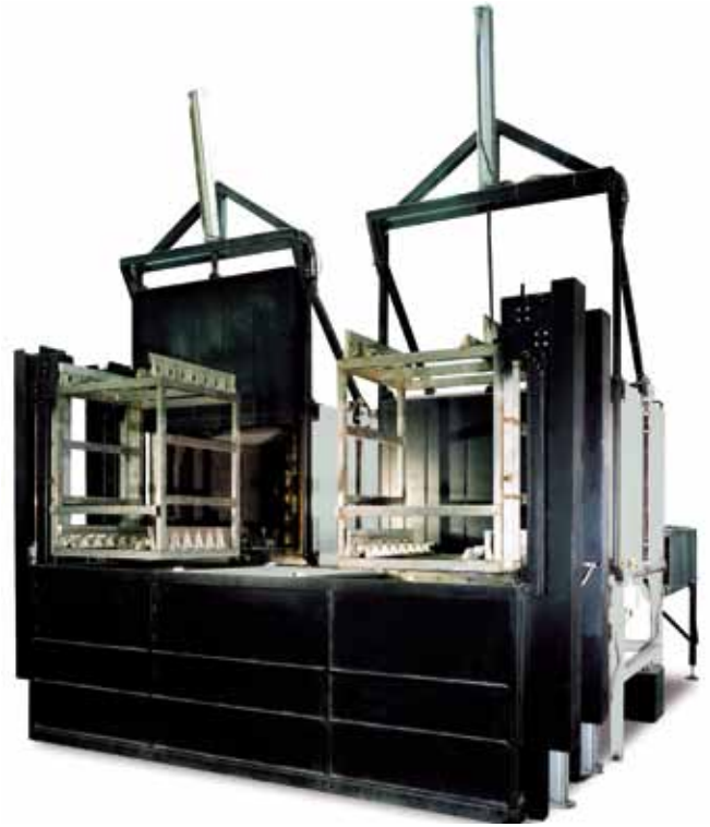
Semi-automatic system Based on two chamber furnaces with integrated quenching baths
