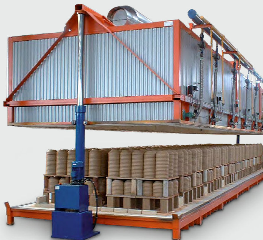
Gas-heated hood furnace for the production of mass-produced goods. The hood is lifted hydraulically
