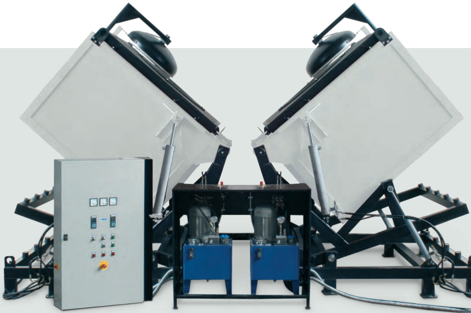
Furnace system consisting of 2 identical tilting crucible furnaces equipped with special hydraulics and control for very fine dosing of the pouring quantity
