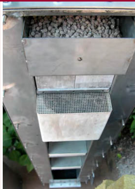
Photos left: : Catalytic exhaust system, individually designed for process- specific exhaust gas quantities and components
