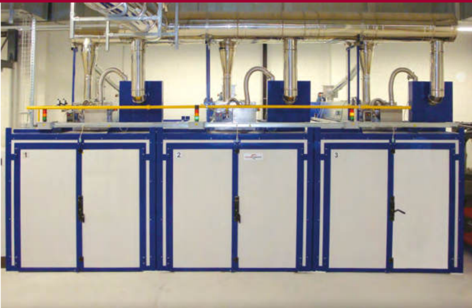
Photo left: 3 indirect gas-heated fur- naces for drying ceramic filters before sintering in a gas-heated sintering furnace.
