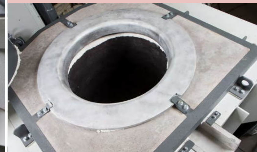
Photo right: Spout in the tilting axis for precise pouring stream Photo below: Cast iron ring to protect the crucible rim
