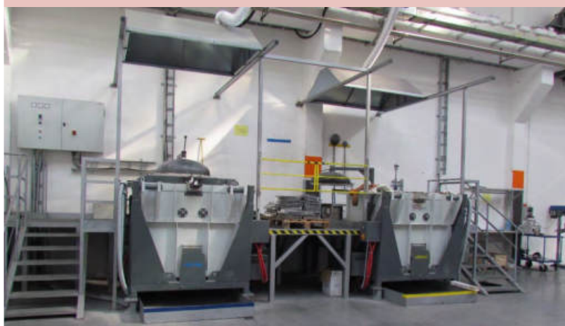
Production line consists of 2 x TA 600/12/K, adjusted working- and charging-platform as well as sliding exhaust bonnets
