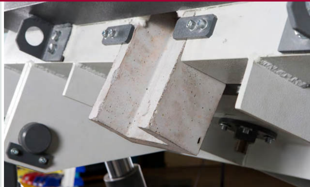
Photo right: Spout in the tilting axis for precise pouring stream Photo below: Cast iron ring to protect the crucible rim
