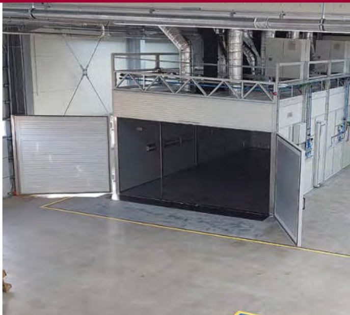
Photo left: 3 indirect gas-heated fur- naces for drying ceramic filters before sintering in a gas-heated sintering furnace.
