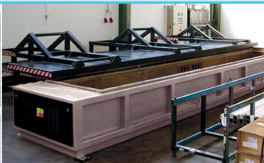
Single-chamber top loading furnaces for preheating aluminium profiles before bending.
