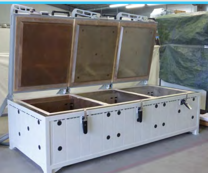
Top loading furnaces with 3 separately controllable chambers for preheating components for shrink-fitting.
