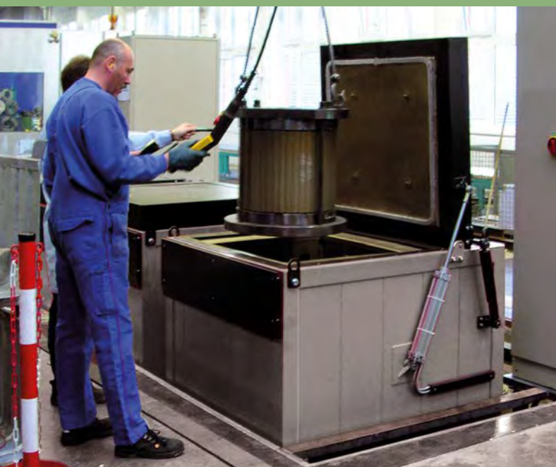
Production plant consisting of 4 top loading furnaces for drying and stoving paints.
