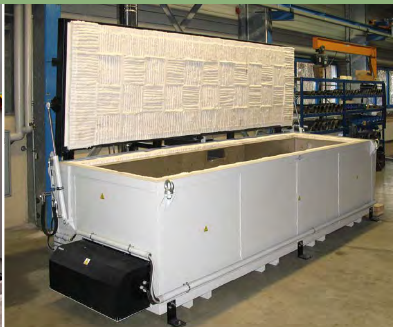
Indirectly gas-heated top loading furnaces with horizontal air flow for tempering plastic-coated rolls for paper production.
