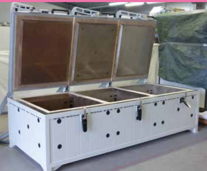
Chest furnace with 3 separately controlled chambers for preheating components for shrink fitting
