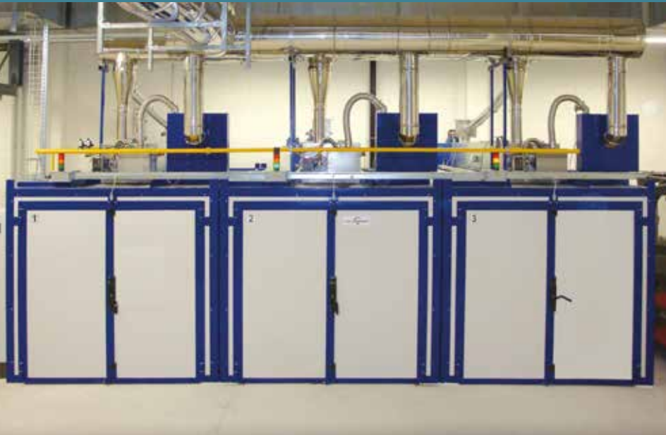
Photo left: Furnace system consisting of 3 indirect gas heated chambers for heat treatment of components up to 150° C.
