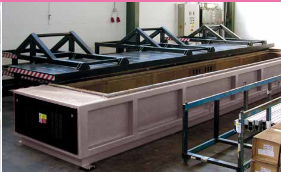
Single chamber shaft furnace for preheating aluminium profiles before bending
