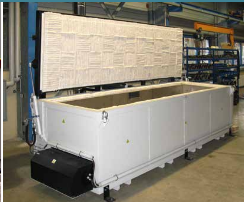
Indirect gas fired horizontal air flow furnace for tempering paper rolls
