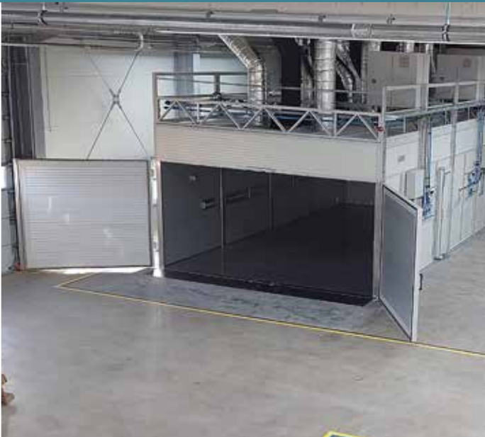
Photo right: 125 m³ low-temperature furnace for working temperatures up to 200 °C, ground level access.
